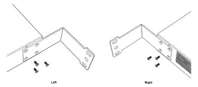
Step 2: Align the mounting holes in the mounting bracket with the mounting holes in the rack, as shown in Figure 3-2.
