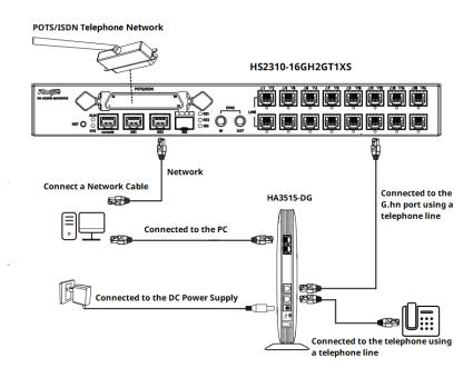
The POTS/ISDN port is connected to the telephone bus.
