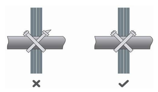
• When cables need to bend, you should first bundle them up. However, the buckle cannot be bundled within the bend area. Otherwise, significant stress may be generated in cables, breaking cable cores. As shown in Figure D-3.
