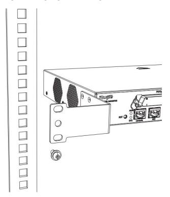
Step 3: Use the supplied M6 screws and cage nuts to securely attach the mounting brackets to the rack, as shown in Figure 3-3.
