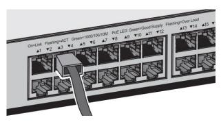
2. Configure the PC with an IP address 192.168.1.xxx. Please note that 192.168.1.200 is in use by the switch.
