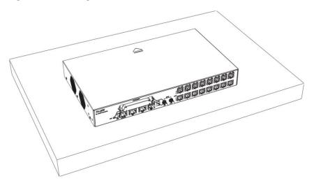
The device must be installed and operated in the place that can restrict its movement.
