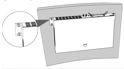
A SUITABLE FOR MOUNTING ON CONCRETE OR OTHER NON-COMBUSTIBLE SURFACE ONLY.
